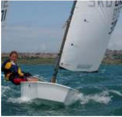
The whole problem of boat balance is compounded by the fact that the mast is unstayed and not only bend backwards and forward but also laterally as well. A rig filled with wind will be forced over the side of the boat so the result is to increase the separation of the opposing forces, the boat will want to screw into wind. This is often made worse by the sailor letting the dinghy heel and the tendency to luff into wind made greater.
